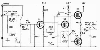
Schematic of SA-1 showing one of twoidentical stereo channels. Circuit is equalized for RIAA playback; output of unit is push-pull.
