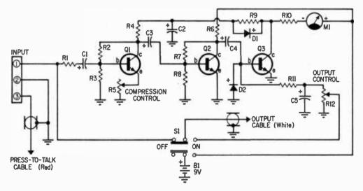
More than just a diode clipper, the C-577 begins to compress the audio signal at -45 db.
