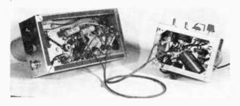
Several sets of patch cords like these are good for making temporary connections while checking newly constructed or modified equipment. A few feet of lamp cord, with an alligator clip soldered to each end of each wire is all that's necessary. A spot of paint can be added for colorcoding so you can match up the correct clips at either end.
