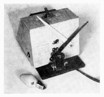
Light shining through chassis apertures from an outside light source energizes the photocells sufficiently to provide enough energy to give transistors a quick check. The only circuit component that might fail is the light bulb which is replaced easily enough. Otherwise, once the tester is set there should be no need for further adjustment.
