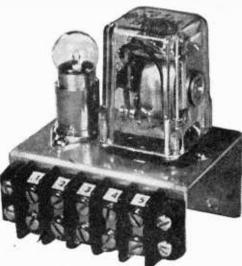
The cold weather car starter can be easily mounted in your engine compartment in the most convenient location. Then just make the five connections to terminal strip TS1.
