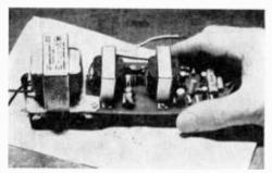
Also, capacitors C4 and C5 are very high in capacity. With the two transistor amplifiers pulling 8 milliamperes of current, R6 can only drop the output voltage 2 volts. No 60cycle hum is heard with a high capacity filter network. A 2200-ohm resistor, R7, is a stabilizing resistor and helps lower the B+ voltage to 12 volts.
