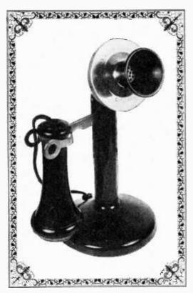
The new has been added to the old in this novel desk stand mike for the ham shack or tape recordist. As shown in the photo, a desk stand telephone of yesteryear has had its old carbon transmitter replaced with a brand new crystal mike cartridge. If you don't have one of these old telephones around, they are still available at some second hand stores, antique dealers, auctions, or from the firms listed in the footnote below.
