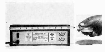
Width of amplifier is 101/4". At left are seen AC cord, and switched AC receptacle. At right are input sockets. Input impedance for phono is 47,000 ohms; for tuner or tape it is 250,000 ohms. AC power drain is 5 watts.
