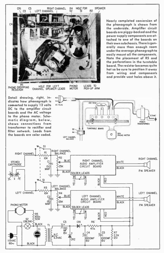
transformer is located. You will then keep all AC components away from the crystal input, eliminating possible hum pickup.
