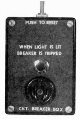
a circuit breaker box to use between the suspected appliance or circuit and the wall outlet. The availability of circuit breakers in low current ratings for TV sets brought the project to completion.
