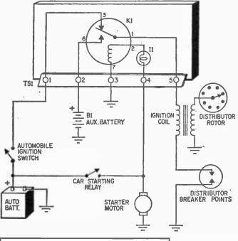
Combination schematic diagram and pictorial shows the car starting aid and its connections to your automobile starting and ignition systems. Current through the starter motor connects the auxiliary battery to the ignition coil through relay K1.
