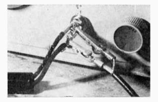
Hooking up that extra pair of headphones for a visitor to the radio shack is done quickly this way. Unscrew the insulating cap from the regular phone plug and add the second pair of phones in parallel using a pair of clips. It's handy for an amateur field day or other contest when an assistant monitors to hear information for the log book. This method may also be used for quickly connecting your receiver to a tape recorder when you want to make an off-the air recording.
