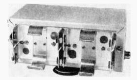
vided for it in the side of the case using epoxy or some other suitable cement. Again, take care that the jack is centered in the hole in the case, and that it does not touch the sides of the hole at any point. Now mount the two battery clips using 4-40 hardware. STAND-BY-OFF switch S1 is mounted in its proper position on the front panel.
