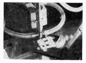
The components are positioned on the substrate, above, to form a complete microcircuit for the Solid Logic Technology module.
