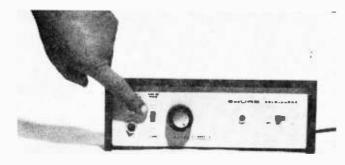
Switch on SA-1 front panel is used to select phono or high-level inputs such as tuner tape. Knob or to riaht. is dual-type control for stereo balance and volume. Although fully transistorized, the SA-1 has selfcontained power supply for operating from 117 VAC. Audio output power is 20 milliwatts; more than ample for listening on headphones.
